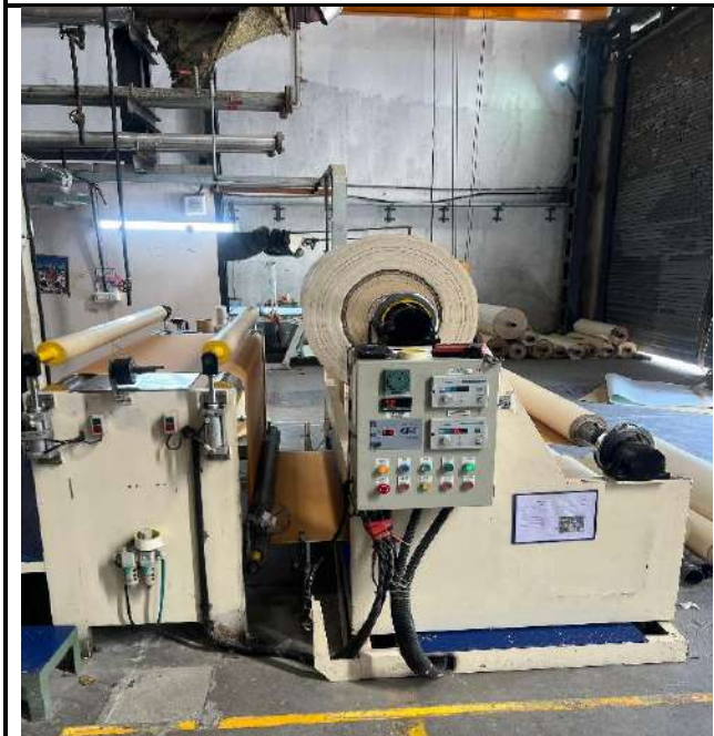
Machinery Name: Unwinder Location In Plant: Main Plant Use: Unwinding Release paper
