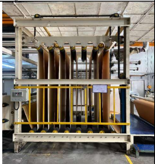
Machinery Name: 35m Accumulator Location In Plant: Main Plant Use: To Accumulate paper for continuous Process
