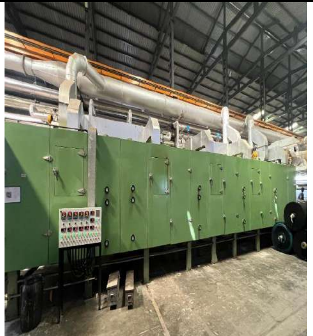
Machinery Name: 15M Oven Location In Plant: Main Plant Use: To make PVC slurry foam to expected thickness or to make PU or PVC slurry dry
